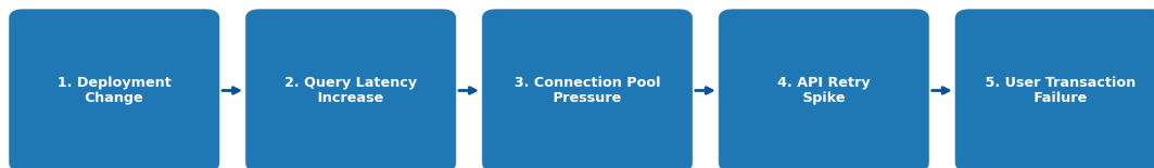
Figure 3. Early Warning Pattern the five signals above (numbered 1–5) as they compound into a single failure path, from deployment change through to user-facing transaction failure.
